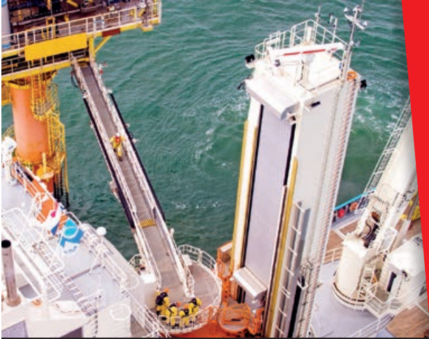
SMST Access & Cargo Tower on board OSV Acta Centaurus
